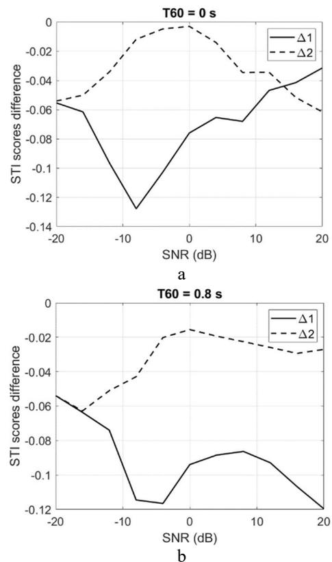
Figure 5. The difference in STI scores for noise (a) and noise plus reverberation (b)
