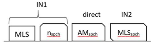
Figure 1. The structure of a multicomponent test signal [12]
