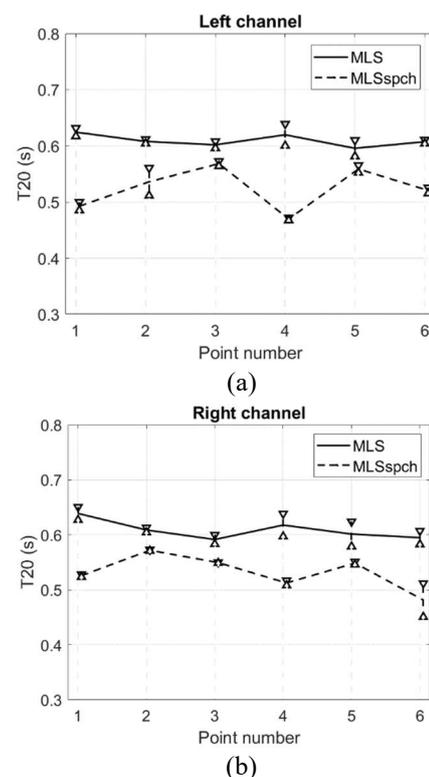
Figure 10. Reverberation time T20 estimates for left (a) and right (b) channels
