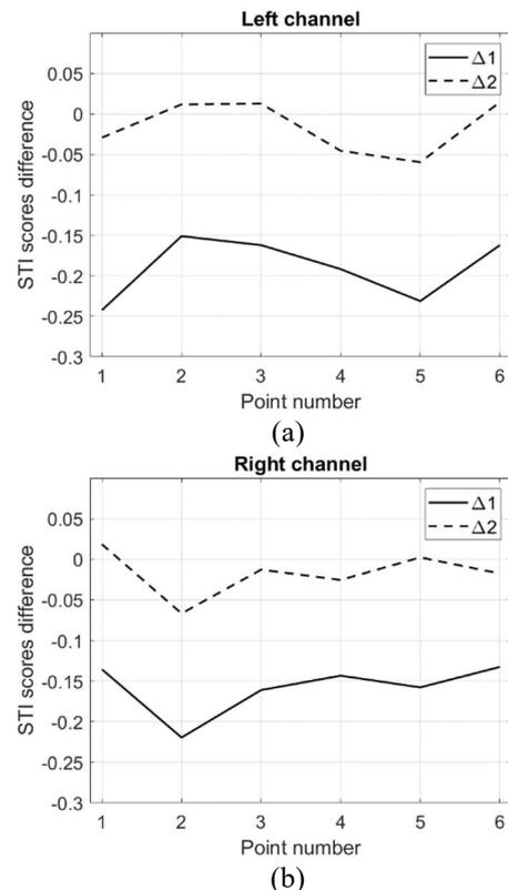
Figure 9. The difference in STI scores in room for left (a) and right (b) channels
